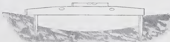
Fig. 72.—STRAIGHT-EDGE AND SPIRIT-LEVEL.
